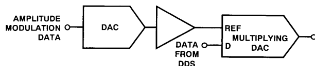
Figure 6. Amplitude Modulation Using a Multiplying DAC
